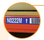
Typical labelling layout for a man-down fork lift application.
